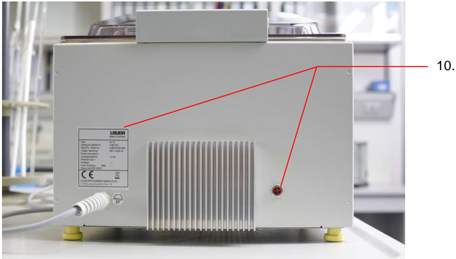
10. Name plate and resetting button for the safety temperature limiter
