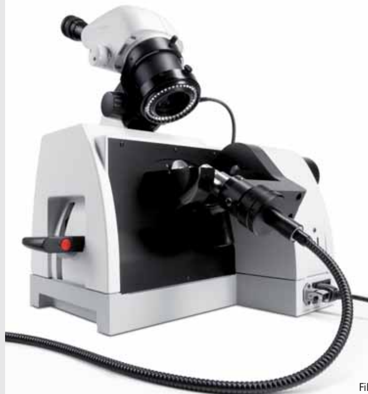
Illumination of the sample during milling
