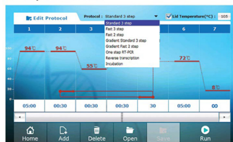
Figure 8. On the 'New Protocol' menu, select a proper protocol among 8 templates.
