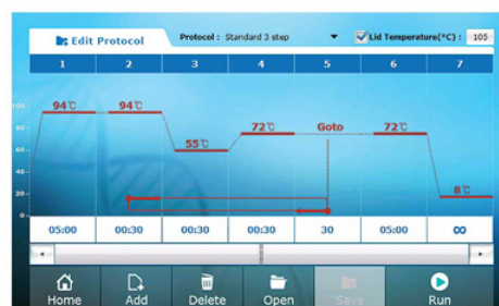
Figure 7. Create new PCR protocols in the 'New Protocol' menu. Make your own protocols by just touching on the screen.
