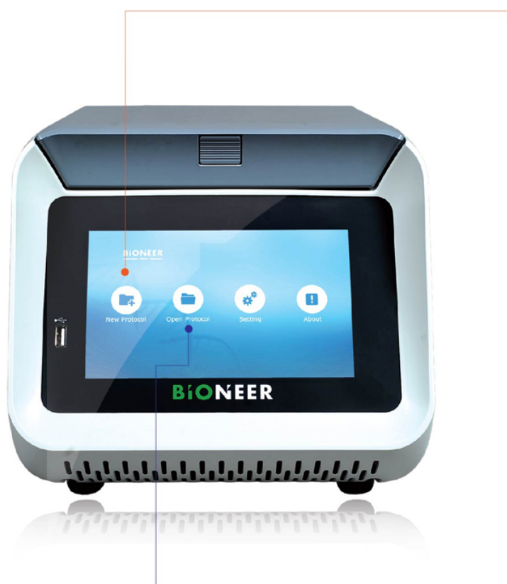
Figure 7. Create new PCR protocols in the 'New Protocol' menu. Make your own protocols by just touching on the screen.
