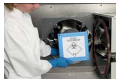
Autoclaving of a HEPA filter cartridge Best-Filter-Protection .
