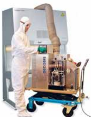
\text{H}_2\text{O}_2 fumigation of a BERNER FlowSafe® safety cabinet with the SKANAIR® DECOSIS system
