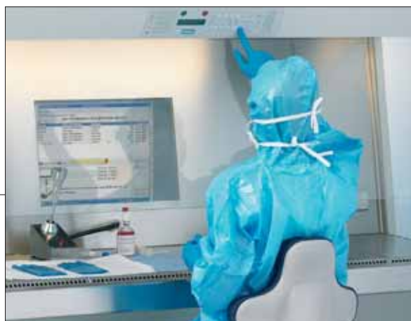
Operating elements within easy reach and displays within field of vision
